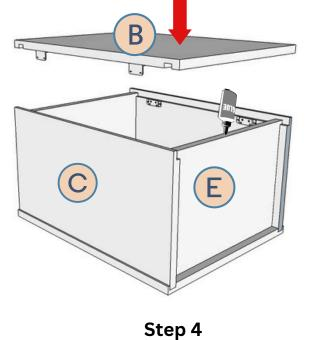
Carefully, turn the cabinet over and tighten the Connector Plate screws holding the Back Panel (B) in place. Lock the plates and L-brackets together using (8)  $\#6 \times 1/2"$  Pan Head locking screws (L).
