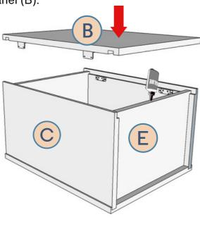
Carefully, turn the cabinet over and tighten the Connector Plate screws holding the Back Panel (B) in place. Lock the plates and L-brackets together using (8)  $\#6 \times 1/2$ " Pan Head locking screws (L).
