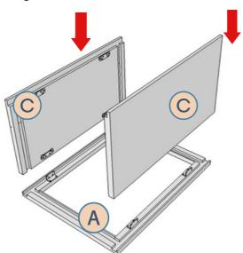
Align the panels so the grooves line up and tighten the Connector Plate Screws. Then, secure the Connector Plates with (8) #6 x 1/2" Pan Head locking screws (L).
