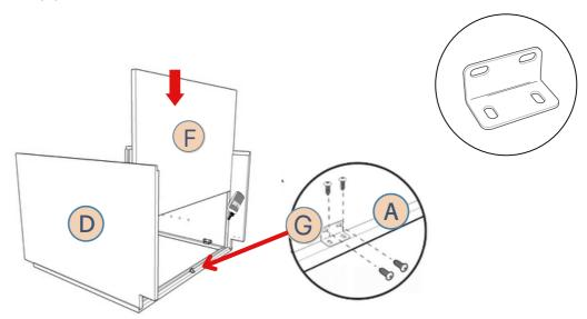
Attach (1) Silver L-Bracket (G) in middle of frame using (4) #8 x 1/2" Pan Head screws.
