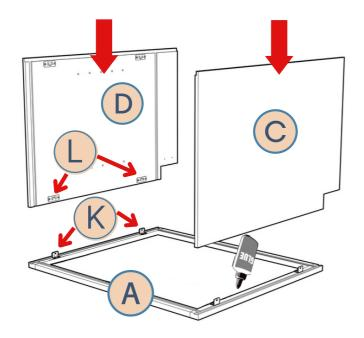
Align the panels so the grooves line up and secure the Connector Plates and L-Brackets with (8) #6 x 1/2" Pan Head locking screws.
