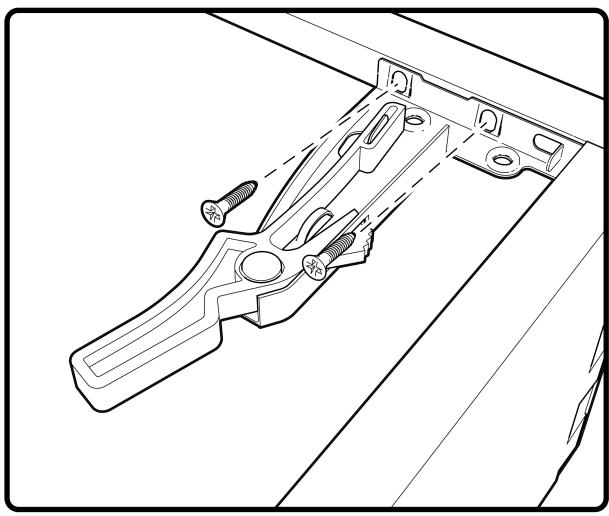
Turn the drawer over and the install (2) Locking Device (V and W), as shown, using (4)  $\#6 \times 5/8$ " Flat Head screws. Do not overtighten the screws
