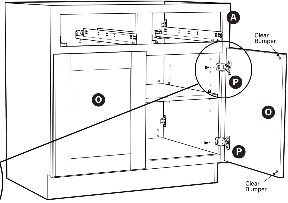
Attach Doors (O) to the Face Frame (A) using (4) #8 x 7/8" Pan Washer Head screws and install (4) Clear Bumpers
