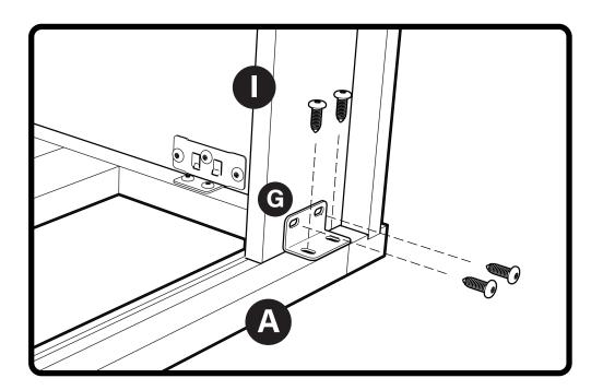
Secure the I-beams (I) to the back of the Frame (A) with (2) silver L-brackets (G) using (8) #8 x 1/2" Pan Head screws.
