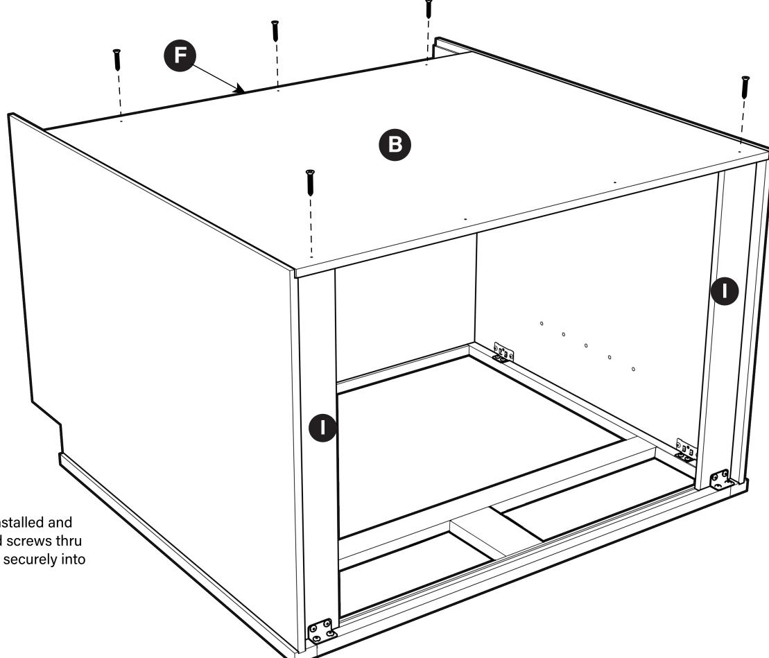
Make sure Back Panel (B) is correctly installed and insert (5) #6 x 1" Countersunk Flat Head screws thru the predrilled holes. Tighten the screws securely into the Fixed Shelf (F) and I-beams (I)."
