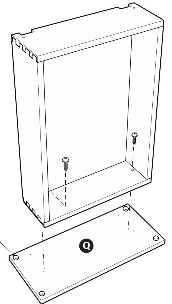
Lay the decorative Drawer Front (Q) face down on a smooth flat surface and install a clear bumper in each corner. If the (2) pilot holes in the back of the Drawer Front are barely visible, we recommend you enlarge them by partially inserting and then removing the attachment screws.
